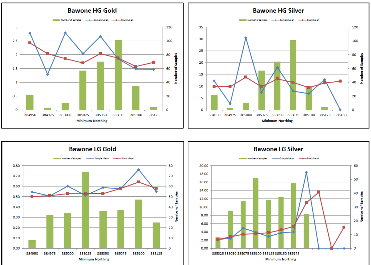
Figure 14-12: Trend analysis for gold and silver in HG and LG Domains, Bawone
