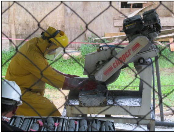
Figure 11-3: Core saw being used at Sangihe.
