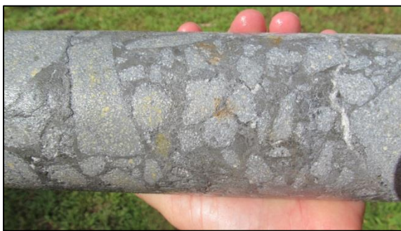
Figure 13: Hydrothermal breccia at Binebase Drill hole BID131_21.67-21.96 m.
