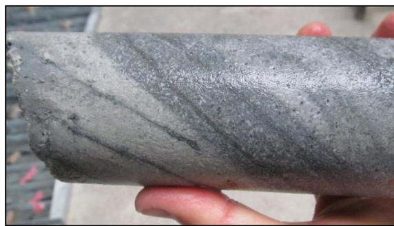
Figure 14: Dacite flows in Binebase Drill hole BID130_50.41-50.70 m.
