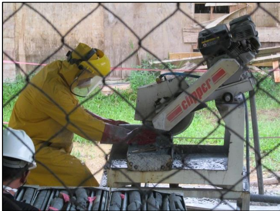
Figure 39: Core saw being used at Sangihe.
