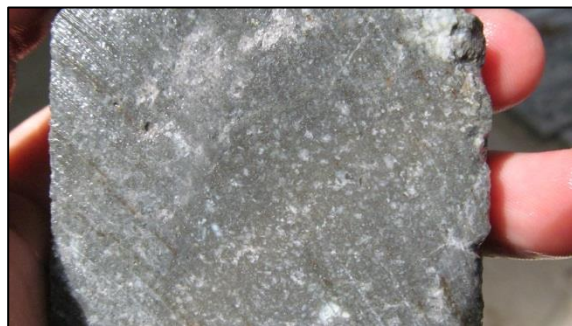
Figure 14: Dacite flows in Binebase Drill hole BID130_50.41-50.70 m.
