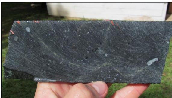
Figure 13: Hydrothermal breccia at Binebase Drill hole BID131_21.67-21.96 m.
