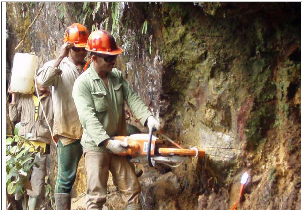
Photo 7: Channel sampling using rock saw (Source: East Asia)
