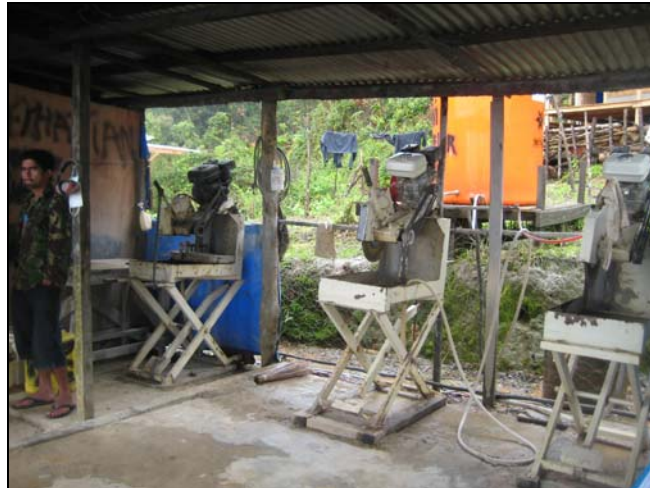
Figure 32: Core Saws (Dimas 5.5HP gasoline-powered diamond core saw)
