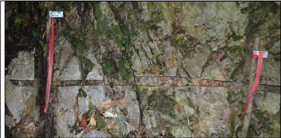
Photo 8: Example of rock-sawn channel sample from outcrop of residual vuggy silica alteration at Miwah Bluff (Source: East Asia)
