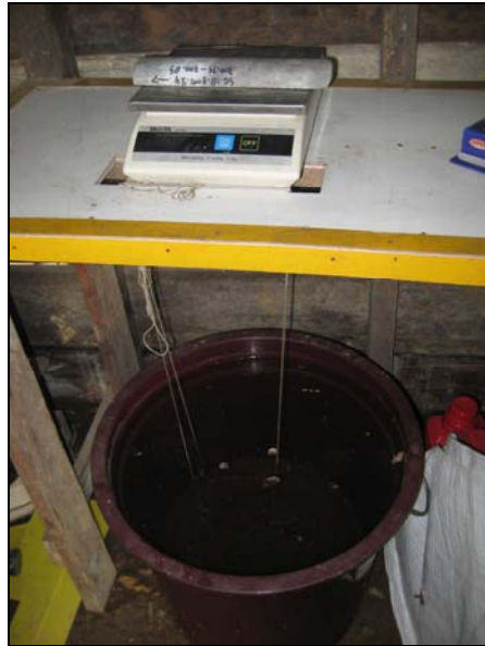
Figure 33: Weighing Core for Immersion Method
