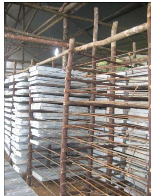
Figure 31: Core Storage shed
