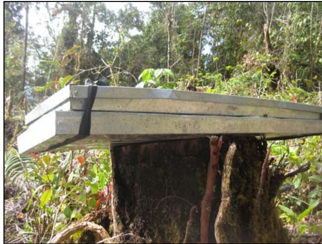
Figure 29: Strapped core tray ready for porting to the core processing facility
